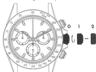
To screw the crown back down against the case, return it to position 1 and apply light pressure on it while screwing it down clockwise against the case.
