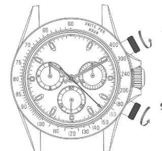
Starting and stopping the timing (Position 1)
