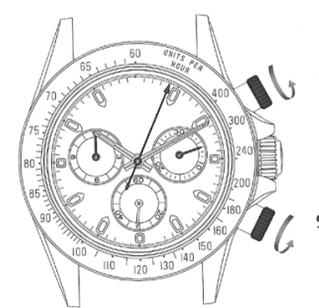
Starting and stopping the timing (Position 1)
